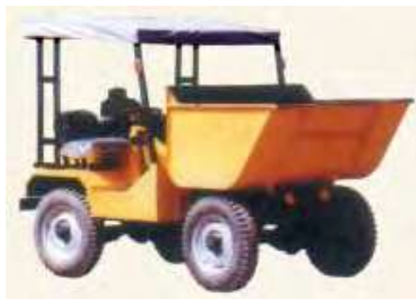
Tough Rider for transporting concrete.
