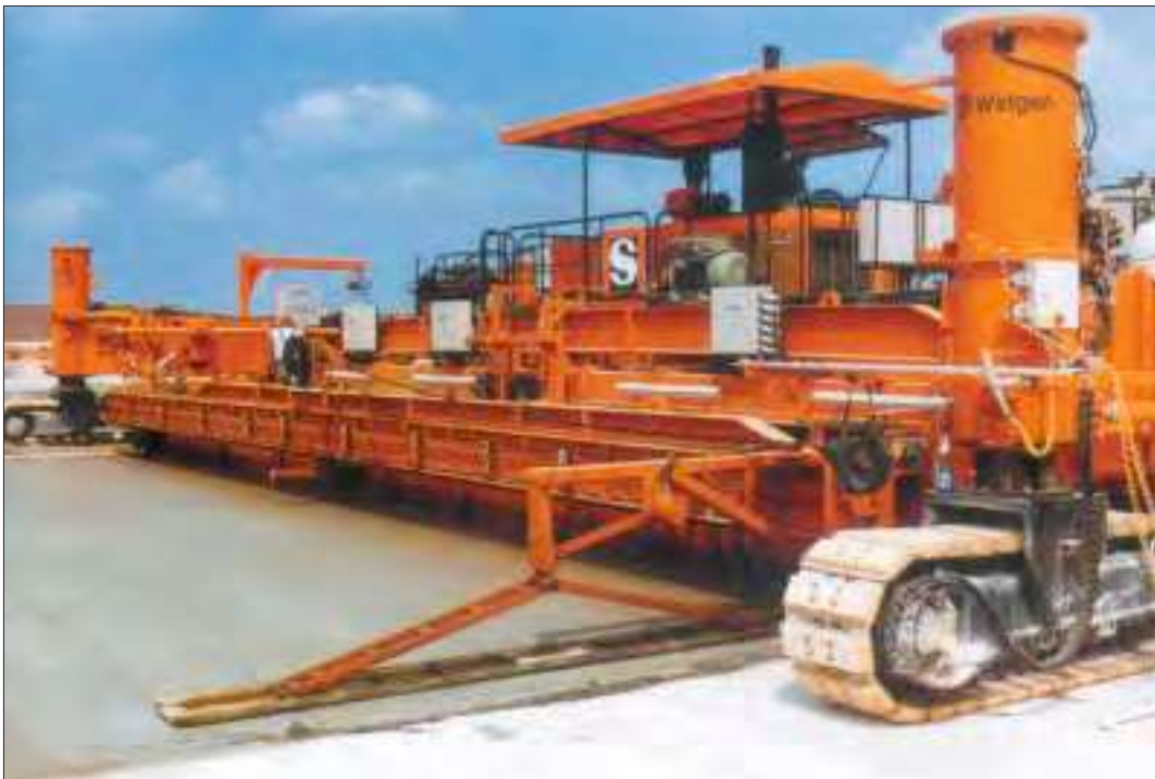
Finishing of road pavement
