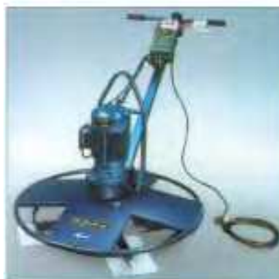
Mechanical trowel for finishing factory floor. Sometimes surface hardener is sprinkled and finished.
