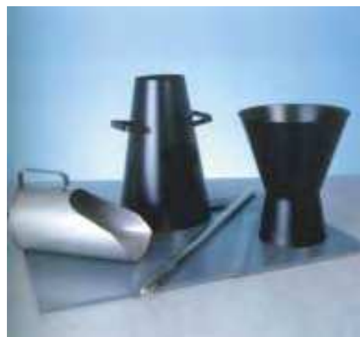
Slump Test Apparatus
