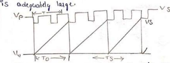
⇒ Also the Sweep voltage is fund to make one cycle for Every two cycles of the synchronising pulses. ⇒ After Synchronism has been Established The of period of the generator decercages stightly 1.8, TS < TO
