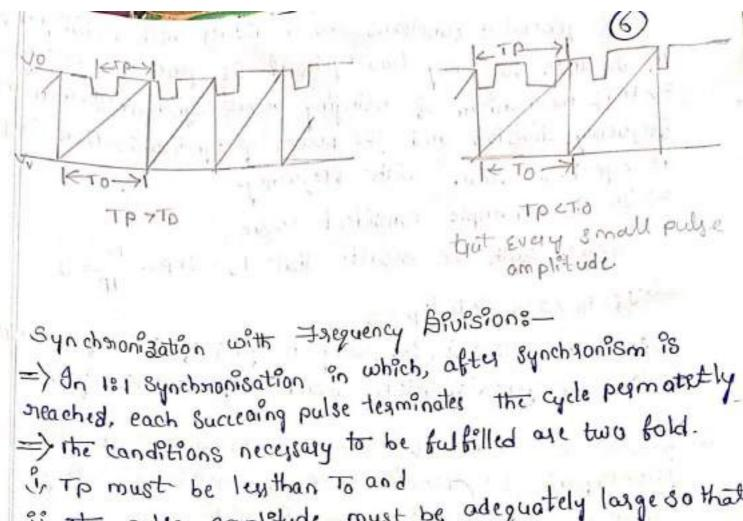
is, the pulse amplitude must be adequately large so that it is capable apable of terminating the cycle permaneterly near the peak. => het us consider the situation when To is much larger than Tp, as for Example. To 7 2 Tp and the pulse amplitude
