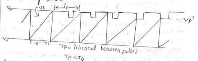
⇒ The application of synchronising pulses, in general, has the Effect of lowering the peak voltage vp. Thus in the figure vp<vp. ⇒ It is seen that the first few pulses have no Effect what aver, on the operation of the generator and the generator contr nuous to run unsynchronised, since these pulses fail to terminate the cycle permatively because of their for adequate amplitude.
