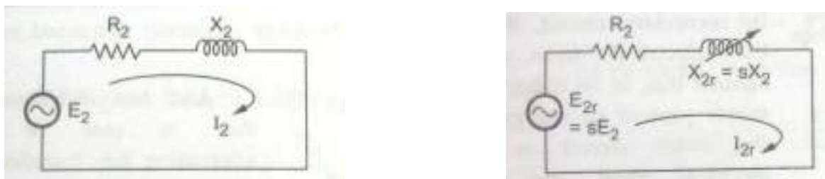
Fig (a): Rotor equivalent circuit at standstill (b): Rotor eq. circuit while running
