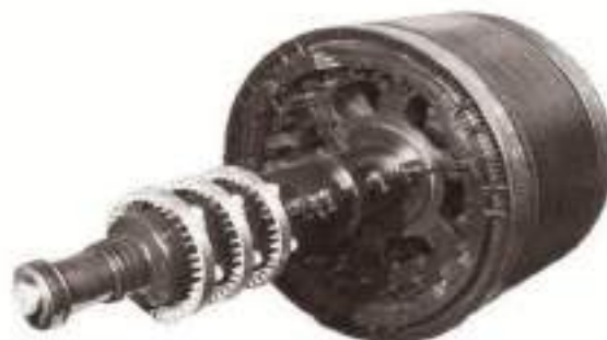
Fig: Typical wound rotors for induction motors. (Notice the slip rings and the bars connecting the rotor Windings to the slip rings)
