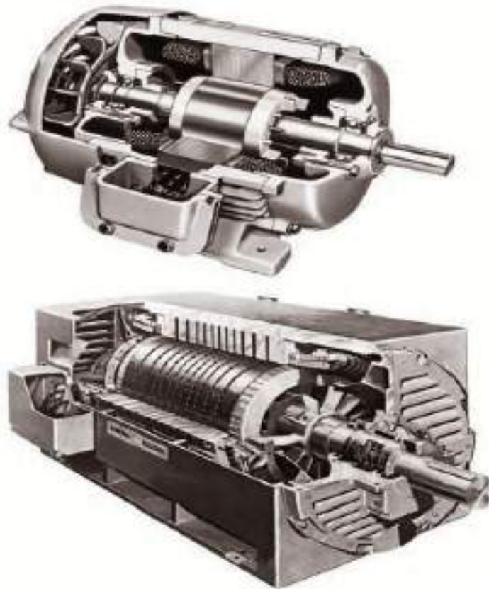
(a) Cutaway diagram of a typical small cage rotor induction motor (b) Cutaway diagram of a typical large cage rotor induction motor.
