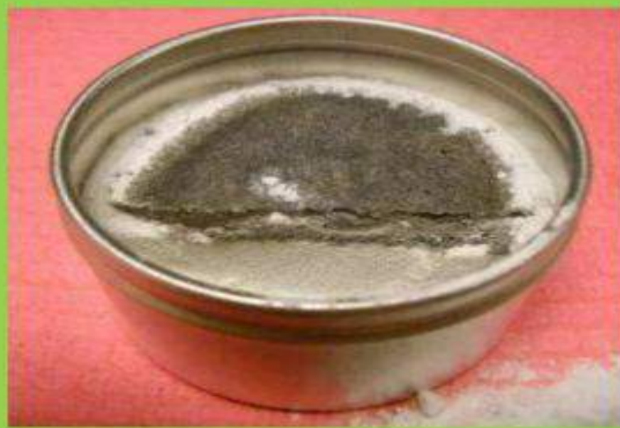
Cross section of the cut specimen depicting the penetration
