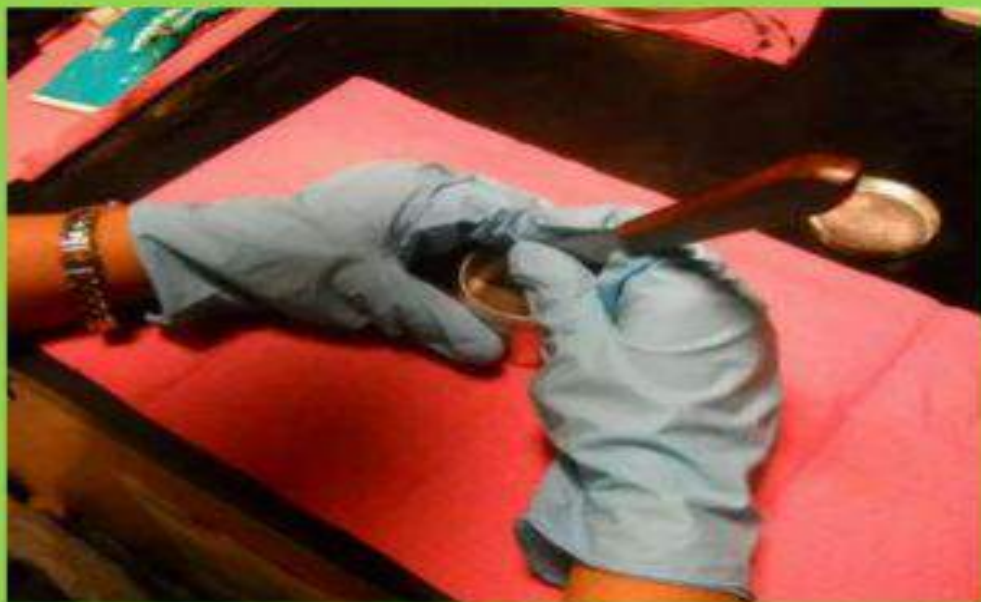
Cutting through the surface of the specimen to determine penetration depth
