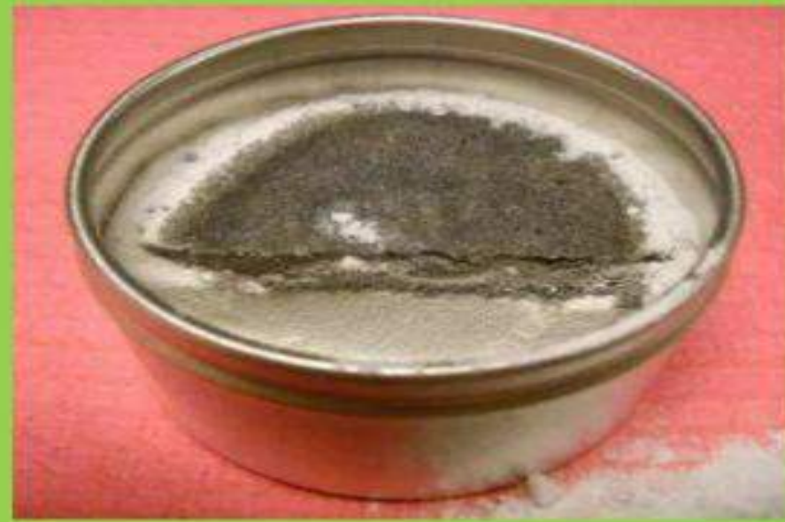
Cross section of the cut specimen depicting the penetration
