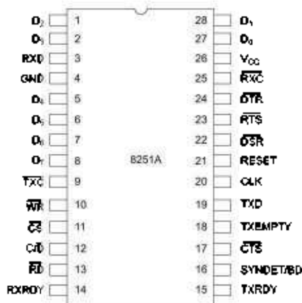
Fig. 6.27 8251A Pin Configuration
