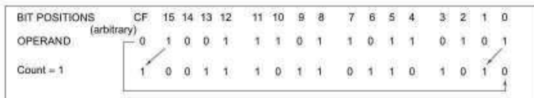
Fig. 2.13 Execution of RCL Instruction
