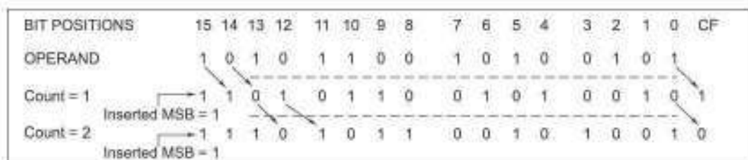
Fig. 2.9 Execution of SAR Instruction
