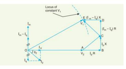
$(I_m - I_q) R$  in phase with  $I_m$  $(I_m - I_a) X$  in quadrature leading with  $I_m$ and From the vector diagram, the relation between  $V_1$  and  $V_2$  is given by ;  $OE^2 = (OA + AB - DE)^2 + (BC + CD)^2$ or  $V_1^2 = [V_2 + I_p R - (I_m - I_q)X]^2 + [I_p X + (I_m - I_q)R]^2$ From this equation, the value of  $I_m$  can be calculated to obtain any desired ratio of  $V_1/V_2$  for a
