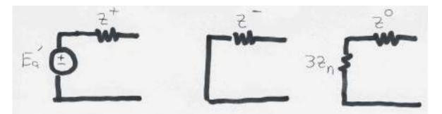
During a fault  $Z+Z^1+Xd^{n}$ . The zero sequence impedance is usually substantially smaller. The value of Zn depends on whether the generator is grounded
