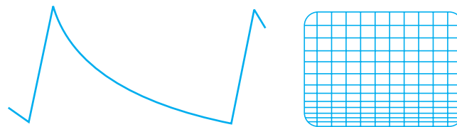
Fig. 19.3 (b). Non-linear sawtooth causing crowding of lines at the bottom of the raster.
