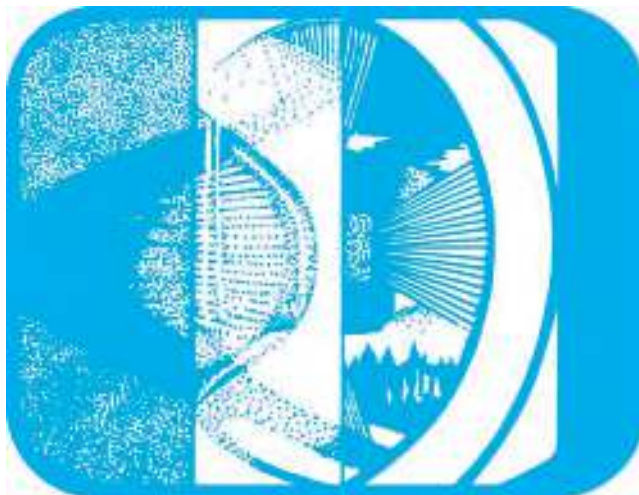
Fig. 30.5. Horizontal foldover at left side of the raster.
