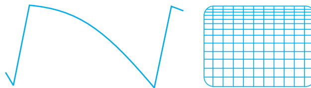
Fig. 19.3 (c). Non-linear sawtooth causing crowding of lines at the top of the raster.
