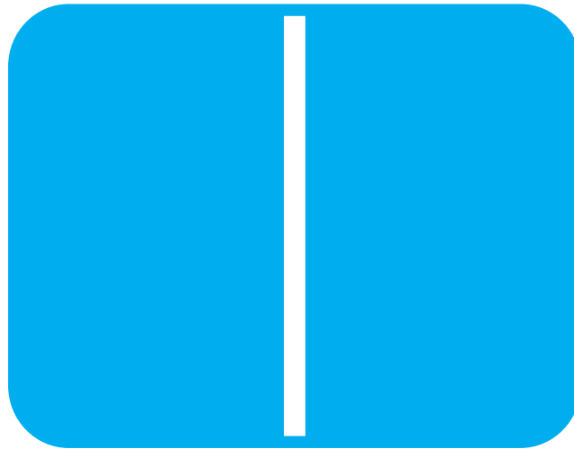
Fig. 30.4. Single vertical line in the centre of the raster due to failure of horizontal sweep circuit.
