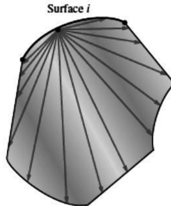
Fig. 6.4 Radiation leaving the surface i of an enclosure intercepted by completely by the surface of enclosure
