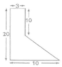
14.A) Find the Area moment of inertia of a T-section as shown in figure.
