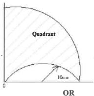
B) Locate the centroid of plane areas shown in the figure. All dimensions are in cm
