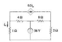
ii) Determine the current Io in 1 Ohm resistor of the circuit shown
