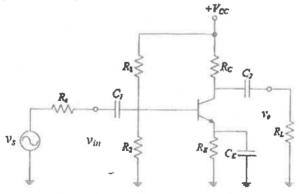
Draw the equivalent circuit and determine  $R_{in}$ ,  $R_{out}$ ,  $A_{v}$ ,  $A_{i}$ .
