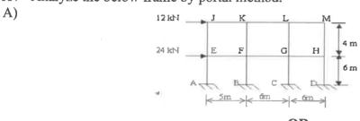
Analyze the frame shown in fig by cantilever method.
