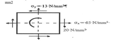
after stressing. Poisson's ratio = 0.3, modulus of elasticity = 200 kN /
