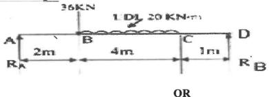
B) Draw shear force & bending moment diagram for the beam shown in CO2 L3 10M fig. 3. & define point of contra-flexure.
